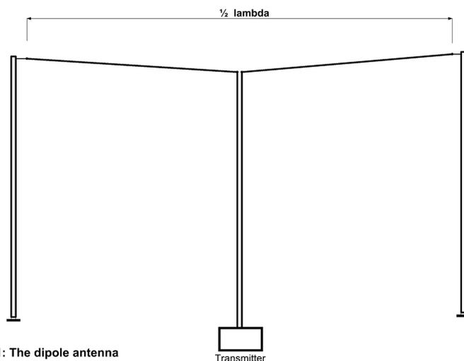
Figure 1: The dipole antenna
