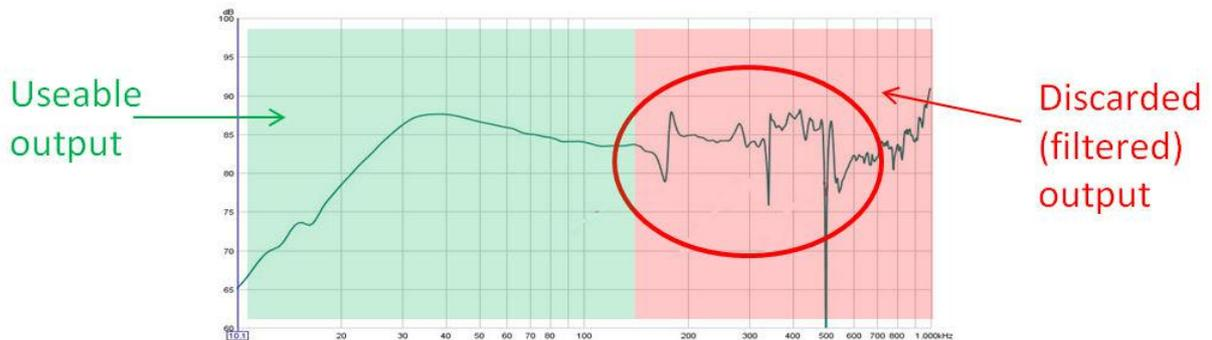
**Figure 5. On-axis response of cone diaphragm speaker. Only part of the frequency range is useable, the region where breakup occurs (red) must be filtered away.**
