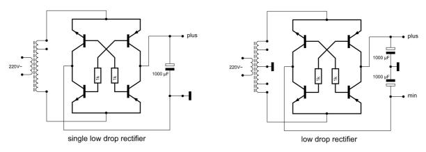
The diagram speaks for itself. The value of the two resistors depend on the  $\beta$  of the transistors and the voltage in question. The transistors should be switching transistors, because of the low knee voltage, to say of no more than 0.2 volt.
